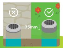
Overflow relief gully must be at least 75mm above surrounding ground level.
