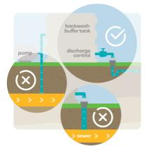
Pool backwash rate must be limited to no more than 0.5 L/s. A buffer tank or pump with restrictor can achieve this.
