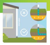
Downpipes must be connected to stormwater, not the sewer. A qualified plumber can check this using a smoke or flow test
